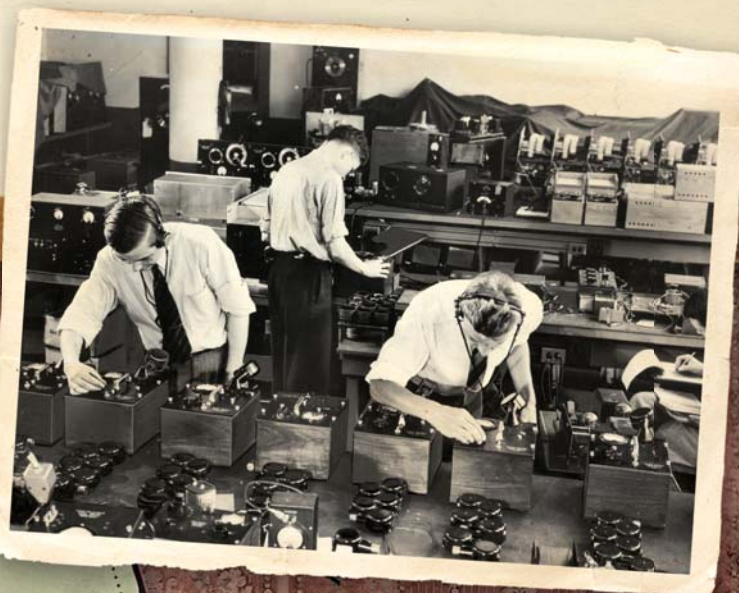
(1938) Co-op students calibrate precision condensers at General Radio. Photo courtesy of Northeastern University Libraries, Archives and Special Collections Department
